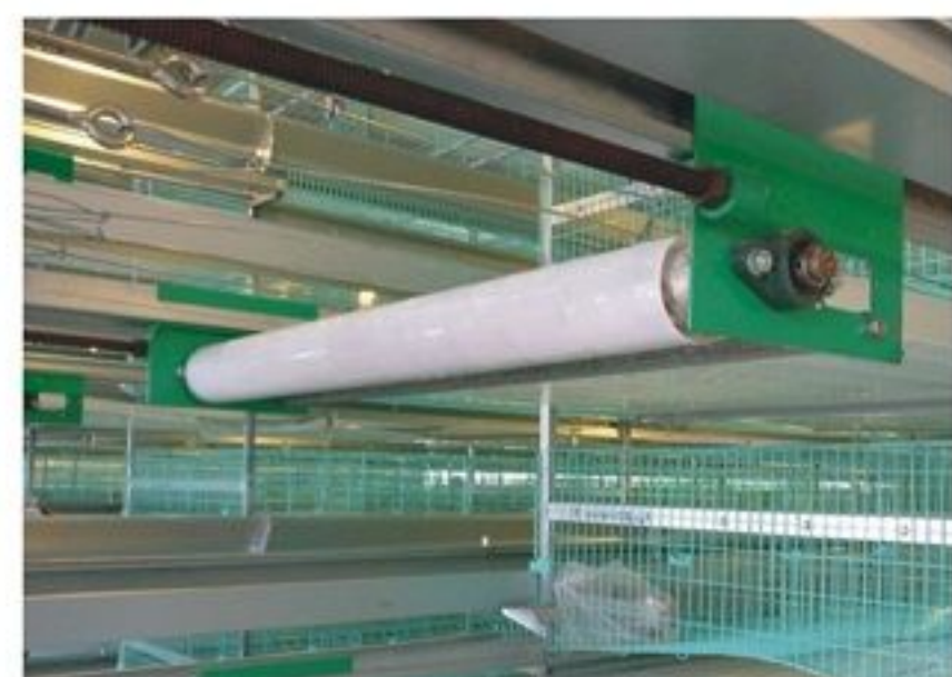
manure conveyor belt
